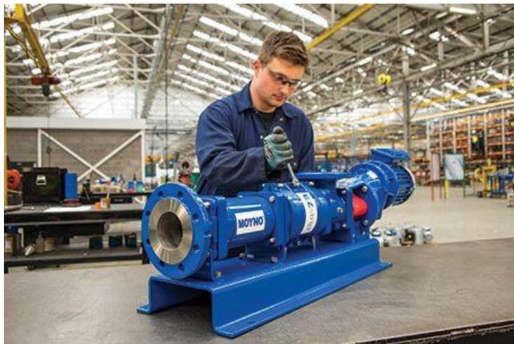
The EZstrip™ maintain-in-place progressing cavity pump from NOV is designed with new features to make maintenance more user friendly. It has quick and safe removal of the full drive train including rotor, stator, shaft, rod and seal. With its patented Positive Torque Split Coupling Rod, maintenance and assembly times are reduced. The tie-bar-free design allows the EZstator clamps to lock the stator securely in place, further reducing stator removal time by over 50% and improving safety of
